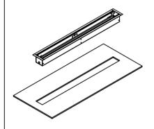
STEP THREE: REMOVE LENS ON FIXTURE. PLACE FIXTURE INTO HOLE CUTOUT IN SHEETROCK. PRESS ALL THE WAY INTO HOLE UNTIL THE BACK FACE OF THE SIDE FLANGES ARE SNUGGLY AGAINST THE OUTTER FACE OF THE SHEETROCK. ONCE YOU ARE CONTENT WITH THE POSITION OF THE FIXTURE, USE WOOD SCREWS TO SCREW THRU THE SIDE OF THE FIXTURE INTO THE 2X4 THAT WAS PREVIOUSLY DISCUSSED.
